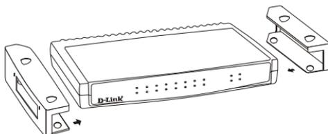
Note when clicking each bracket into place, the round feet on the bottom of the device will line up with the round holes on the bracket. The brackets are designed to fit snugly in place. Please do not force them.
